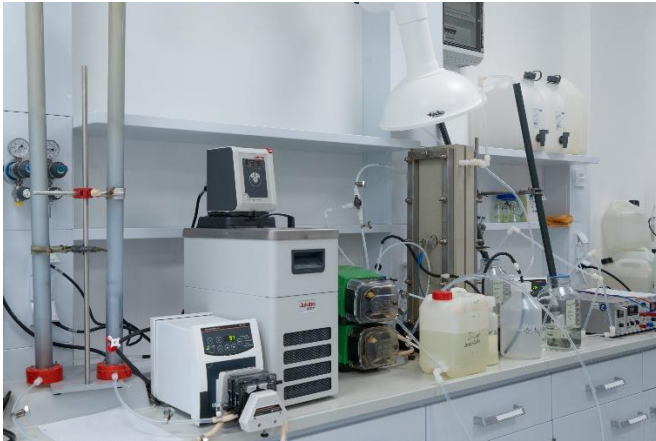
Image 2: Clean production: the lab testing equipment for ecofriendly manufacturing of green soda through bipolar electro dialysis of brine. The process eliminates carbon emissions and salty wastewater.
