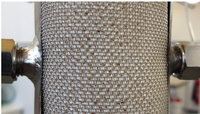
Zeolite granules in a test setup at Fraunhofer IKTS to determine the heat storage properties.
