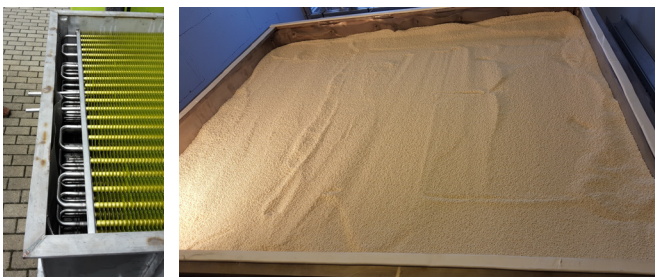
Prototype of a zeolite heat storage tank with 150 kWh storage capacity.
