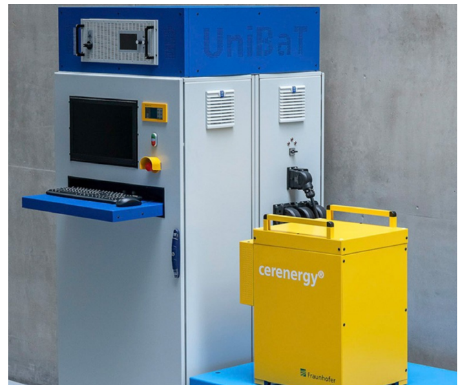
Test stand for analysis of stationary battery modules and systems.
