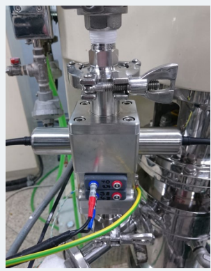
Eddy-current and ultrasonic probes installed on ballmill.
