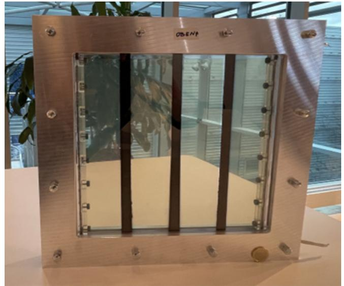
*500 cm<sup>2</sup> single module of a self-sufficient PV-PEC reactor.*
