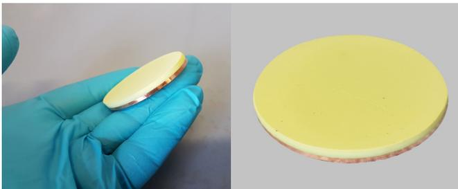
*Cu-bonded WO<sub>3</sub> sputtering target from IKTS for the DC sputtering process (can be used unbonded for RF magnetron sputtering).*
