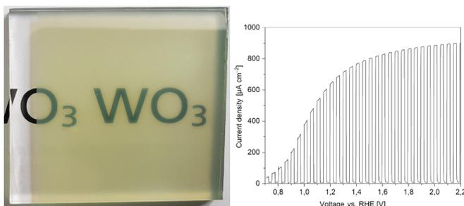
*Transparent WO<sub>3</sub> layer of approx. 1µm thickness deposited by DC sputtering (left), photoelectrochemical activity (right).*
